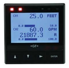
The 9950 Transmitter is a two channel controller that supports two sensors of same or different types in one instrument. The sensor types supported by the 9950 are Signet Flow, pH/ORP, Conductivity/Resistivity, Salinity, Temperature, Pressure, Level, Dissolved Oxygen, and devices that transmit a 4 to 20 mA signal with the use of the 8058 iGo® Signal Converter.
