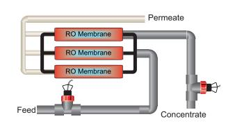
% Recovery C: [(Feed - Concentrate) ÷ Feed] × 100 In the Setup menu, select the option that states % Recovery C, FEED: CONC
