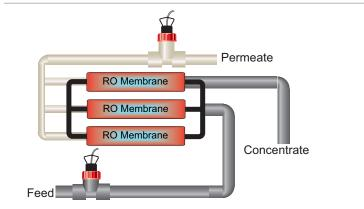
% Recovery A: (Permeate ÷ Feed) × 100 In the Setup menu, select the option that states % Recovery A, FEED: PERMEATE
