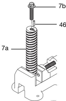
**FIG. 15: Prepare the Shaft (7a) for Assembly**
