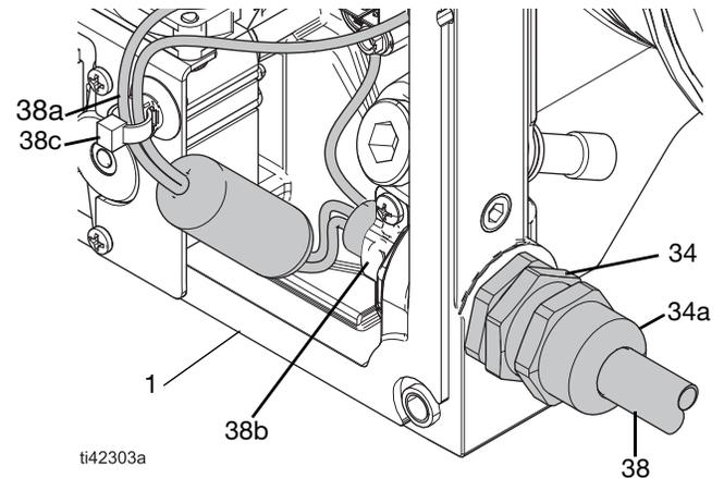
**FIG. 4: Power Cord/Cable (F-2 and F-4 motors)**
