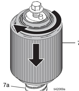
**FIG. 16: Assemble the Shaft and Rotor**
