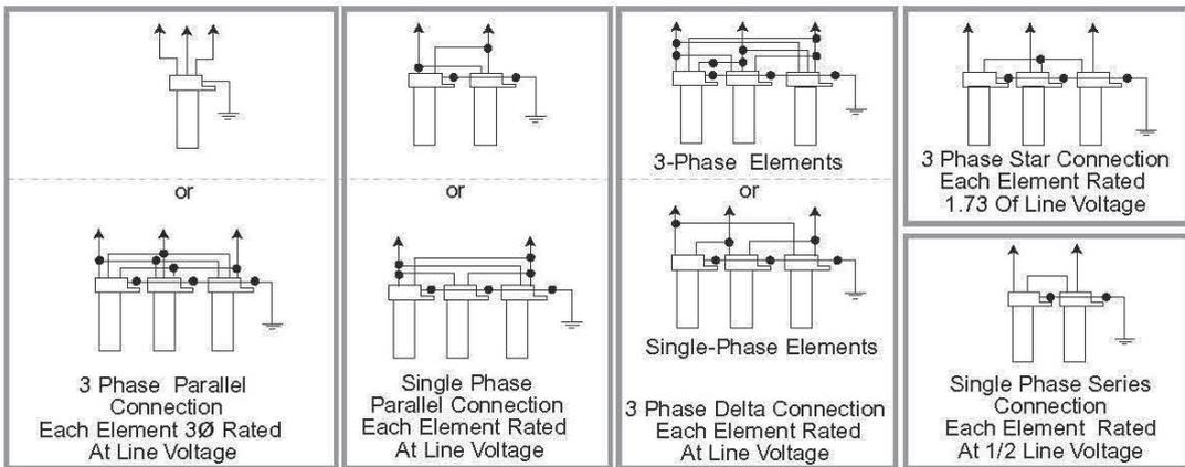
**Figure 2** Single and Three Phase Connection Wiring Diagrams
