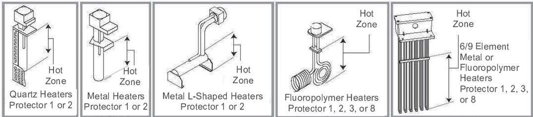
**Figure 1** Typical Heaters and their Over Temperature Protectors
