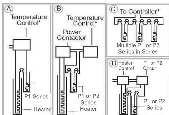
\*Temperature control requires reset circuitry for Protector 2 Series operation.
