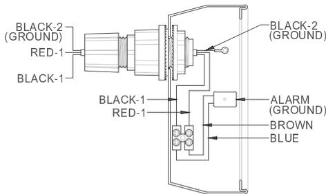
**SINGLE ALARM WIRING DIAGRAM**
