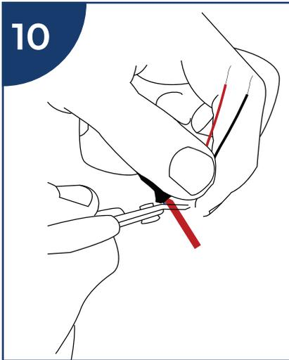
10 Cut the capillary tube on an angle
