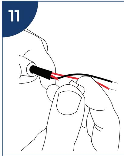
11 Put the filter back on the capillary tube after cut
