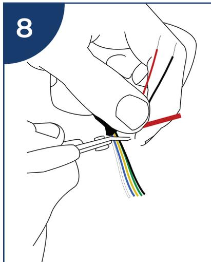
6 Cut off the remaining coloured wires
