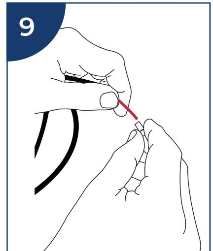
7 Take the filter off of the capillary tube after the cable is cut
