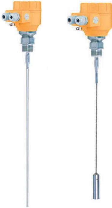
The 2291 Guided Wave Radar level transmitter is designed for continuous level measuring of conductive or non-conductive liquids, pulps and solids. The 2291 level gauge operates based on the well-known TDR (Time Domain Reflectometry) principle. Micropulses are sent along a probe guide at the speed of light. As soon as the impulse reaches the surface of the medium, it is reflected back to the electronic module. Level distance is directly proportional to the flight time of the impulse.
