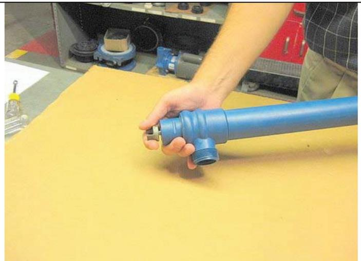
To install the impeller you will need to hold the pumps coupling...
