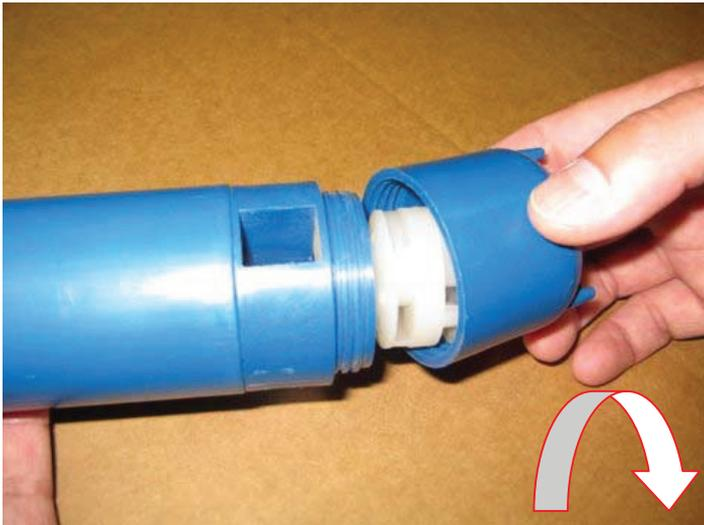
Remove the impeller housing cover by turning it clockwise.
