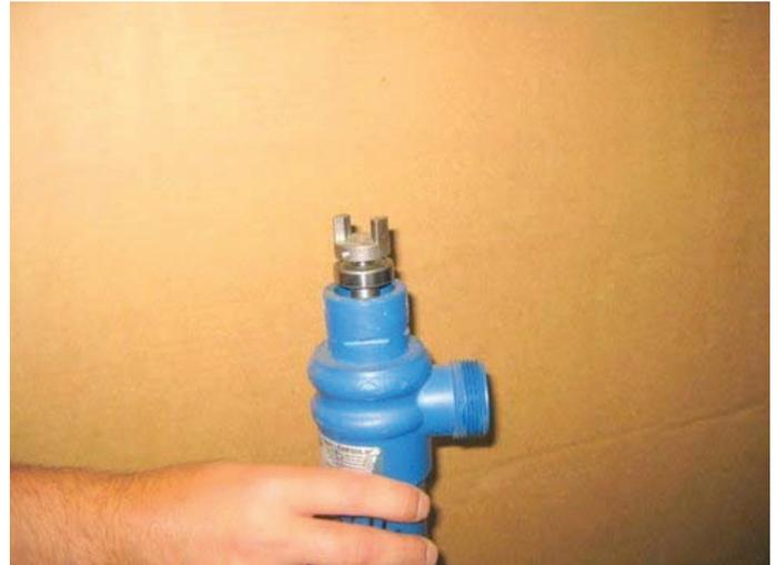
Picture showing bearing assembly partially removed from pump head.
