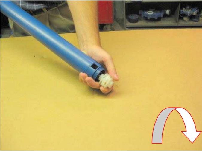
and with your other hand screw the impeller onto the pumps shaft (turn clockwise).
