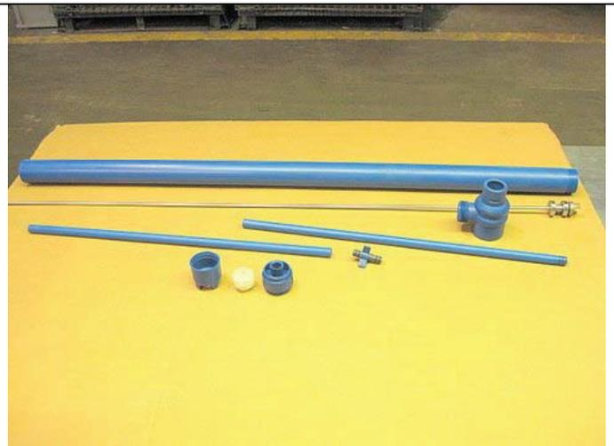
Picture illustrates pump completely disassembled.
