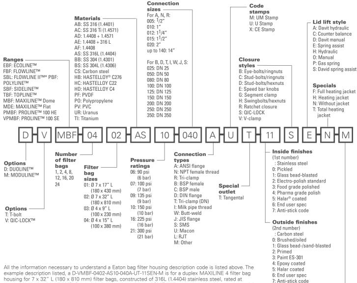
housing for 7 x 32" L (180 x 810 mm) filter bags, constructed of 316L (1.4404) stainless steel, rated at 150 psi (10 bar), with 4" ANSI flange inlet/outlets. It carries an ASME "U" code stamp and has a tangential outlet. The housing has a glass bead-blasted finish both inside and outside, has a QIC-LOCK opening mechanism, a spring-assisted cover lifter, does not have a heating jacket and is a "special" design.
