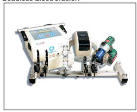
20mm - 63mm (1/2" - 2") Size Range Single wall **Piping** PVDF Plug: 110V **Materials Power** Tool: 230V / 15A 17"x12"x12" **Dimensions** 35 lbs. Weight 48"x40"x37" **Shipping Dimensions** 475 lbs. **Shipping Weight**
