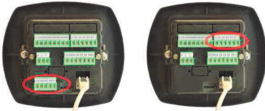
Figure 6-11 - The first 2300 version, shown on left, has two sets of contacts connecting a switch to reset the totalizer on a separate connector (C1-C4). The most recent version has no separate connector for a switch. However, three connectors on the pulse (or "digital") connector can be used as an input for a switch.
